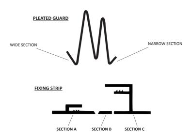
Use a stanley knife to cut the strip into sections A, B and C before commencing installation.
